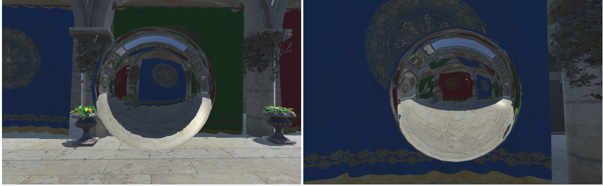
Figure 3.9: Reflections rendered on spherical surfaces in different areas of a scene, using the DTPC technique. The same source cubemap is used, but the result has been parallax corrected so that the correct reflected image appears despite displacement from the sample point. The right hand image shows some evidence of artifacts due to the occlusion failure case.
