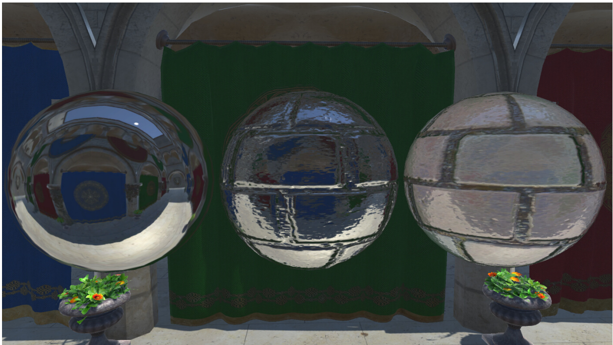
Figure 3.4: From left to right: 1) Basic cubemap reflections. 2) Reflections with the surface's normal vectors determined by a normal map. 3) Reflections with a normal map using Schlick's approximation of Fresnel reflection to determine the influence of surface colour versus reflected colour.
